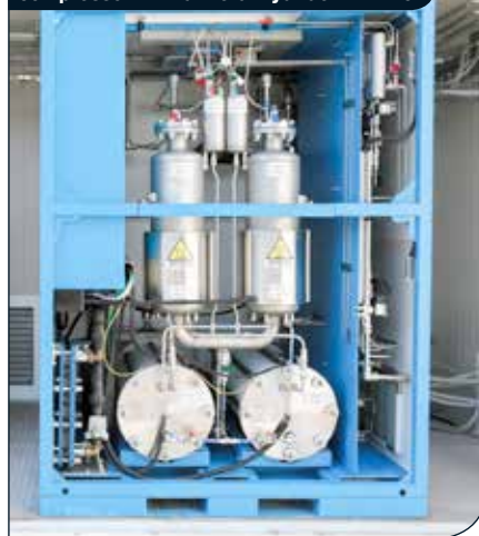
EPFL has developed a hydrogen compressor with a metal hydride ZrMn1.5.
