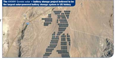
The Gemini project is also using a DC coupled system which uses an electrical configuration designed to add more efficiency and is one of the first DC-coupled solar battery storage systems of its size in the US.
