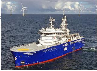
Horizon is a new class of purpose-built SOV with walk-to-work (W2W) capability developed by Damen in consultation with the offshore renewable energy industry and designed to meet the increasing demand for vessels capable of operating in ever further off-shore locations.
